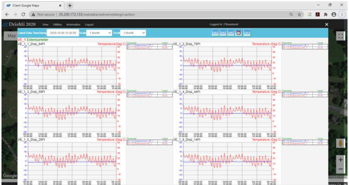
Multipoint Borehole Extensometer data
